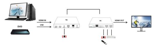
2. the allocation extender (1 to N): all RX ID number adjusted to TX ID, can achieve 1 TX to 255 RX
