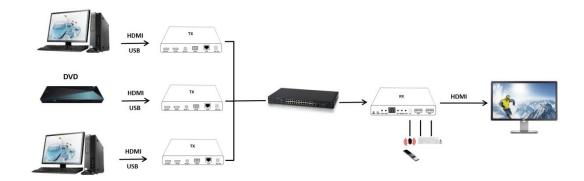
4. Matrix (M to N): by adjusting RX's ID number, switch to different ID TX, to achieve many-to-many mode
