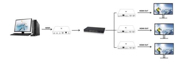
3. switcher (N to 1): by adjusting RX's ID number, switch to the corresponding TX
