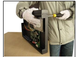
③fix the screw of hard disk
